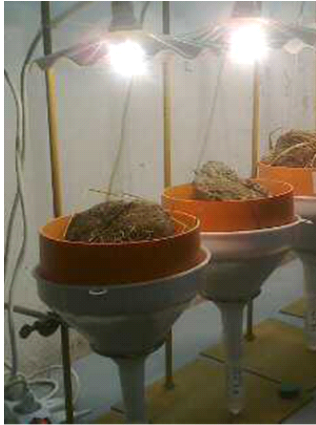
Fig 2 - Microarthropods extraction by modified Berlese-Tullgren funnels.
